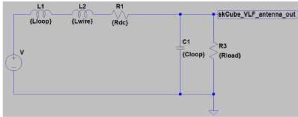
Fig 4. VLF antenna circuit mode
