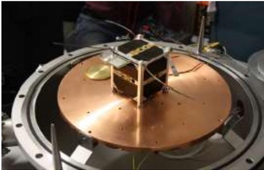
Fig. 1. skCUBE on a vacuum chamber plate at the Institute for Experimental Physics in Košice, shortly before vacuum tests.
