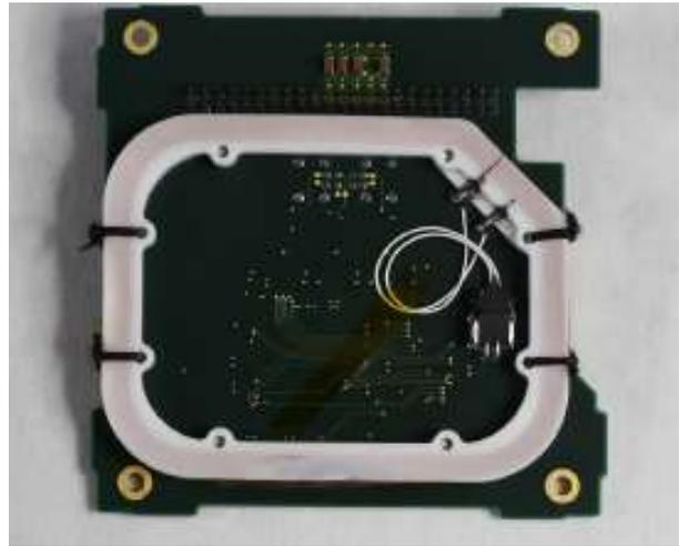
Fig. 3. Power circuit board of the detector.
