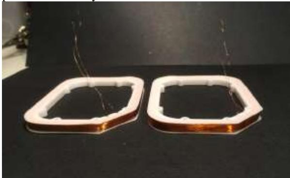
Fig. 2. Two identical coils, of which one was enclosed into a plastic container and attached to the experimental power circuit board of skCUBE.
