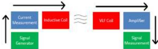
Fig 5. Schematic view of a sensitivity measurement performed on the receiver. Arrows indicate measurement sequence from signal generation, with pre-determined properties, up to its amplification and final detection. The signal generator (PC sound card); current measurement (Fluke 287 multimeter); inductive coil (one loop with a diameter of 25 cm, distance 17 cm from the detection VLF coil); amplifier (OPA2314); signal measurement (Creative X-FI USB sound card).
